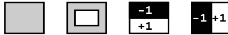
Fig. 1. Zone types used. Two simple statistic zones returning either mean or standard deviation, and two weighted sum zones
